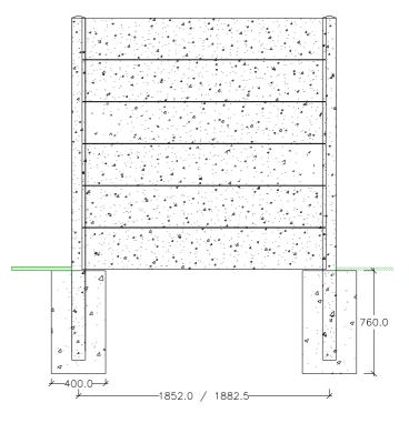
Posts should be buried to a depth of 600 mm in a minimum 400 x 400 mm rectangular or 400 mm diameter auger hole, and backfilled using concrete to a prescribed mix type C15 as described In the "Irish Building Specification,"
