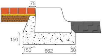
NOTE: IF THE POSSIBILITY OF SEVERE IMPACT IS A PARTICULAR CONCERN T16 BARS CAN BE PROVIDED @ 200 C/C IN THE HAUNCHING CONCRETE GRADE 15N10 MINIMUM
