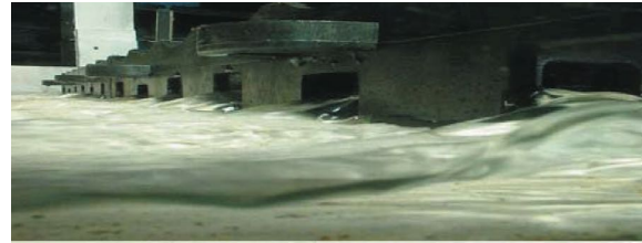
The SCS INEGRA system has the unique benefit of full scale independent physical hydraulic modelling, providing the necessary data for developing validated porous paving designs on a scientific basis.
